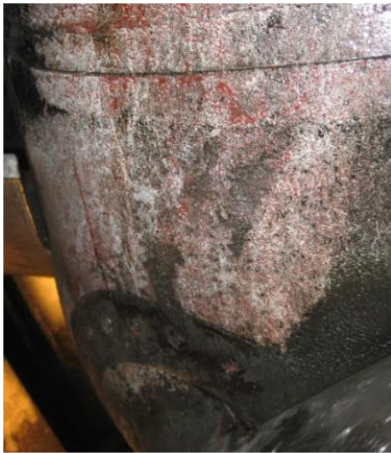
Figure 19. Stainless Steel Overlay on the Blades Suction Side (Underside, Leading Edge)
